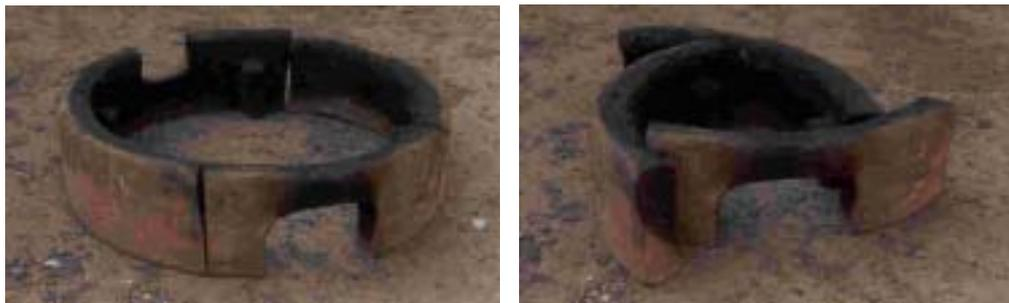
Figure 8: 4Section Gounziye with smoke outlet
